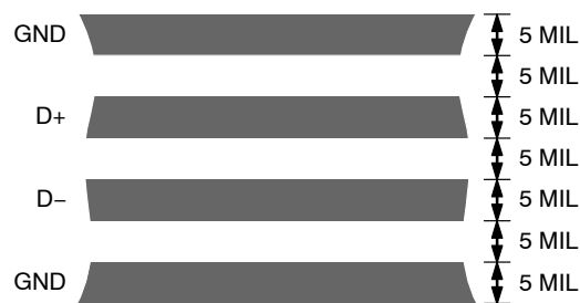
Figure 22. Typical Arrangement of Signal Tracks
