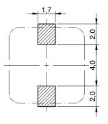
no sensitive traces underneath the component
