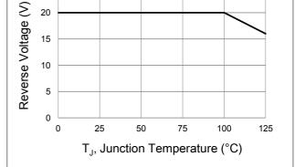
Fig. 4. Operating Temperature Derating Curve
