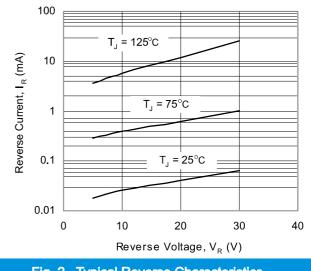
Fig. 2. Typical Reverse Characteristics
