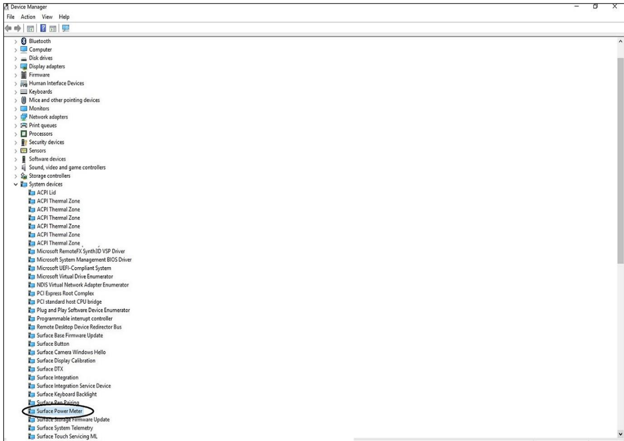
Figure 2. Select Surface Power Meter under System devices.
