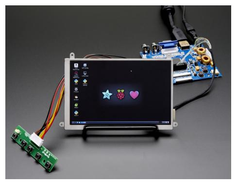
This is our smallest high-res display, with 1280x800 resolution. It's not IPS, however! This version comes with an Audiocapable driver. we also have a version without audio (PID #1666)
