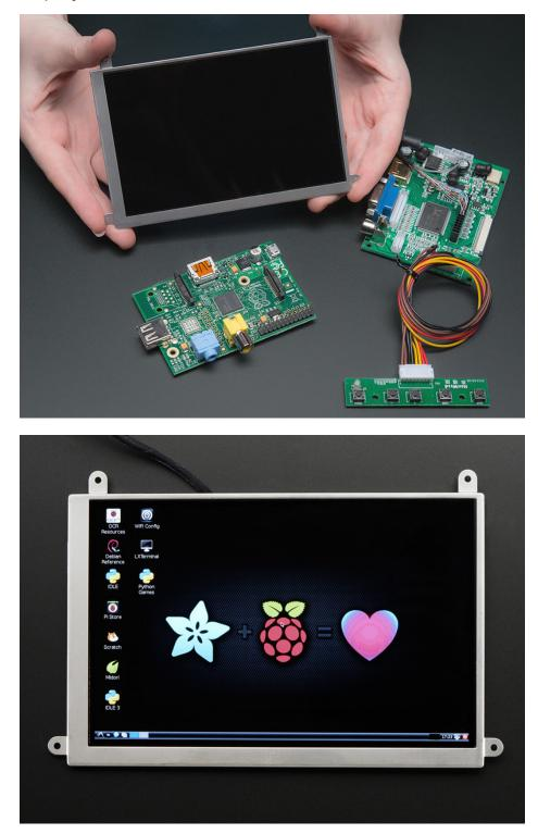
This is our smallest high-res display, with 1280x800 resolution. It's not IPS, however! We also have a version with HDMI audio support (PID #1695)
