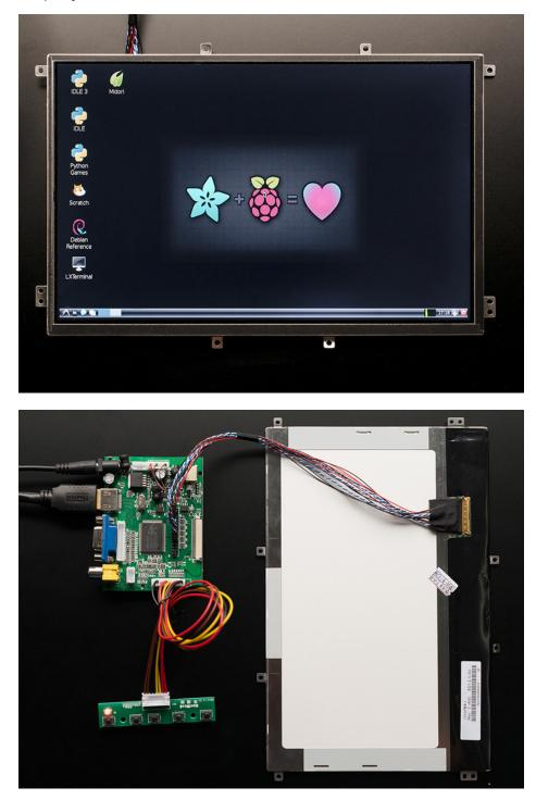
This is one of our prettiest display It's got excellent resolution (1280x800!) and IPS display so it is bright, crisp and looks good from any angle. This driver even has HDMI audio support and can drive two 4 ohm speakers directly.
