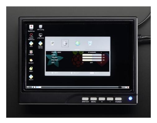
Sound Mode - Standard, Personal, Music, Movie Bass - Adjust the bass Treble - Adjust the treble Balance - Adjust the balance AVC - Off/On - Automatic Volume Control
