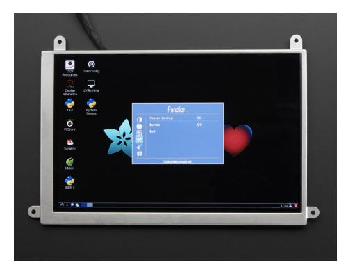
**Power Saving -** 10s to 60s - how long it takes for the screen to shut off **Burnin -** On/Off - a function to prevent screen <u>burn-in (https://adafru.it/dTR)</u>
