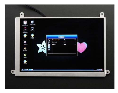
Power Saving - 10s to 60s - how long it takes for the screen to shut offPowertip - no idea what this doesMode: SYS0, SYS1, SYS2, SYS3 - we've found this doesn't effect the image on these displays
