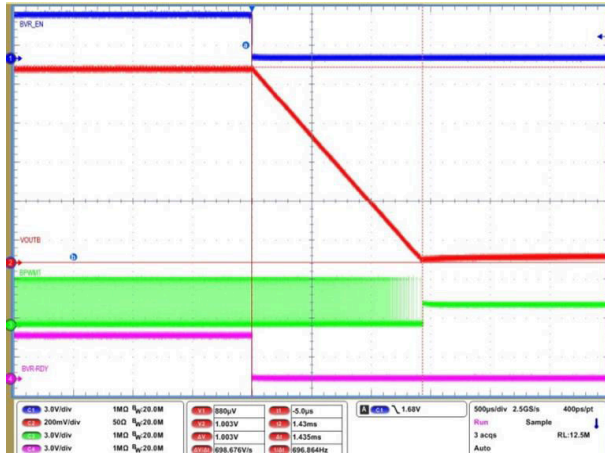
Figure 8-15. Soft-stop channel B (0 ms TOFF_DELAY)
