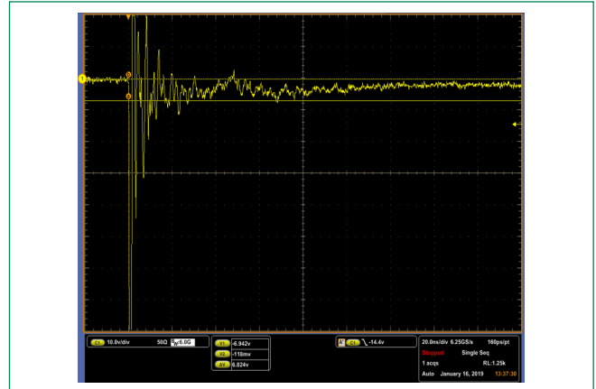
ISO10605 (C:330pF, R:330Ω) contact discharge plot at -8KV
