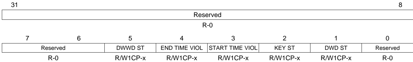
Figure 13-41. Watchdog Status Register (RTIWDSTATUS) [offset = 98h]
