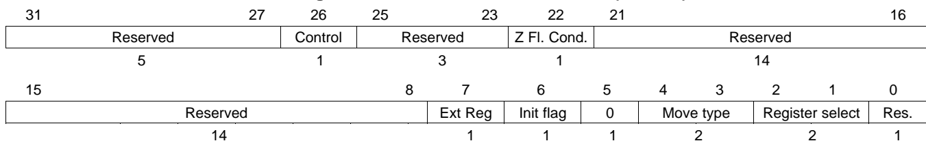
Figure 23-154. MOV32 Control Field (C31:C0)
