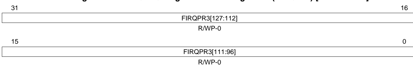
Figure 15-20. FIQ/IRQ Program Control Register 3 (FIRQPR3) [offset = 1Ch]
