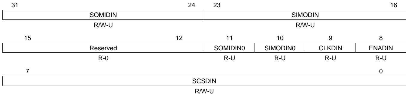
Figure 28-33. SPI Pin Control Register 2 (SPIPC2) [offset = 1Ch]
