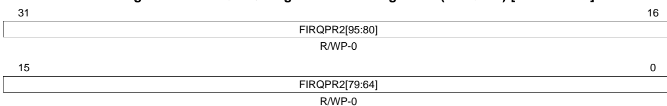
Figure 15-19. FIQ/IRQ Program Control Register 2 (FIRQPR2) [offset = 18h]
